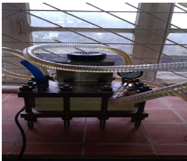
Figure 1. Filter-press type microfiltration experimental apparatus
